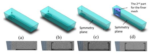
Fig. 4. Mesh with (a) 0.9 million elements, (b) 4 million elements, (c) 8 million elements – symmetry (d) 1.5 million elements – symmetry – 2 parts.
