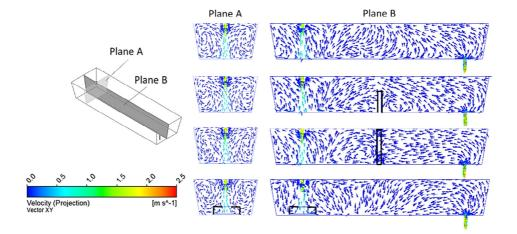
Fig. 5. Velocity flow field of (a) bare tundish, (b) tundish with dam, (c) tundish with baffle and (d) tundish with turbostop.
