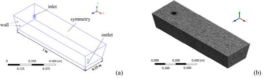
Fig.1. (a) Boundary conditions and (b) mesh elements inside the single strand tundish model.
