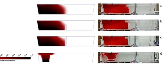
Fig. 9. Tracer flow after 3 seconds of injection in (a) bare, (b) tundish with dam, (c) tundish with baffle and (d) tundish with turbostop.
