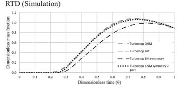
Fig. 11. Residence time distribution (RTD) curves of tundish model with turbostop and different mesh resolution: 0.9 million elements, 4 million elements and 8 million elements – symmetry, 1.5 million elements – symmetry – 2 parts.
