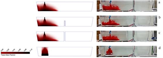
Fig. 8. Tracer flow after 1 second of injection in (a) bare tundish, (b) tundish with dam, (c) tundish with baffle and (d) tundish with turbostop.
