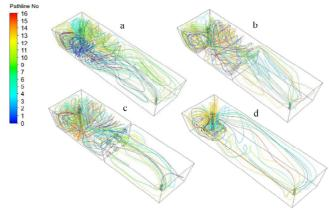
Fig. 6. Streamlines of fluid flow inside the tundish model: (a) bare tundish, (b) tundish with dam (c) tundish with baffle and (d) tundish with turbostop.
