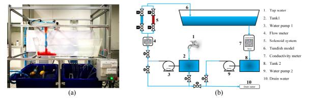
Fig. 2. (a) the physical water model of single strand tundish (b) the schematic diagram of water modeling system setup used to analyze the tracer injection and the residence time distribution.
