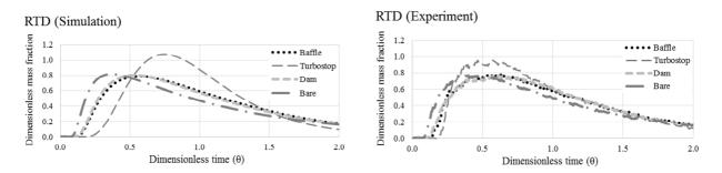
Fig. 10. Residence time distribution (RTD) curves for each tundish model: (left) simulation results, (right) experiment results.
