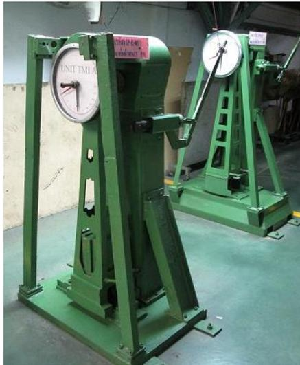
Figure 3.8 Charpy Impact Test Machine
