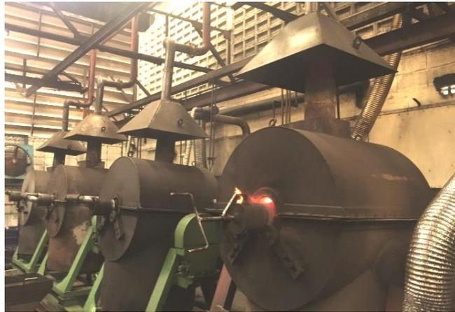
**Figure 3.2 Rotary Retort Furnace**
