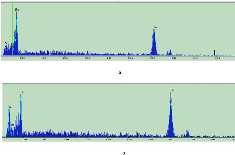
Fig. 12. The elemental analysis results from Energy-dispersive X-ray: (a) Original product, (b) experiment specimen CN-01.
