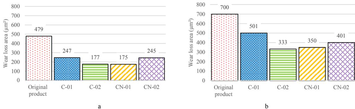
Fig. 10. (a) Wear loss area after 15 minutes; (b) Wear loss area after 30 minutes.
