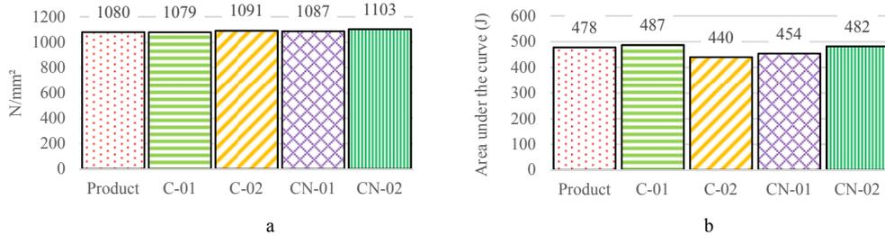
Fig. 9. (a) Shear strength of specimens; (b) Toughness of specimens.
