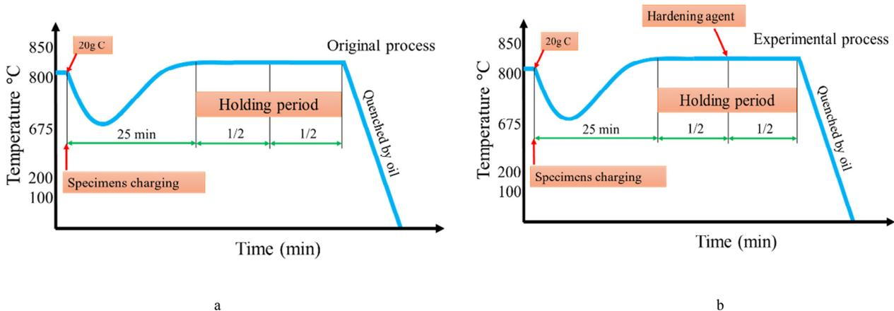
Fig. 4. (a) Original heat treatment profile of the factory; (b) heat treatment profile of the test experiment.
