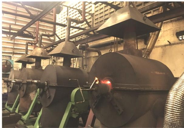
Fig. 3. Rotary retort furnace at the factory.
