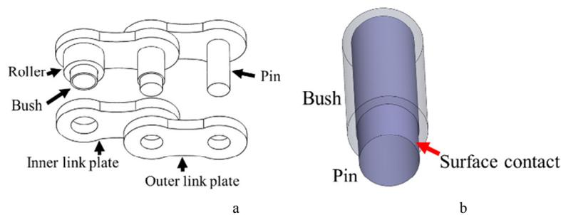
Fig. 1. (a) Assembly of roller chain; (b) The surface contact between pin and bush.
