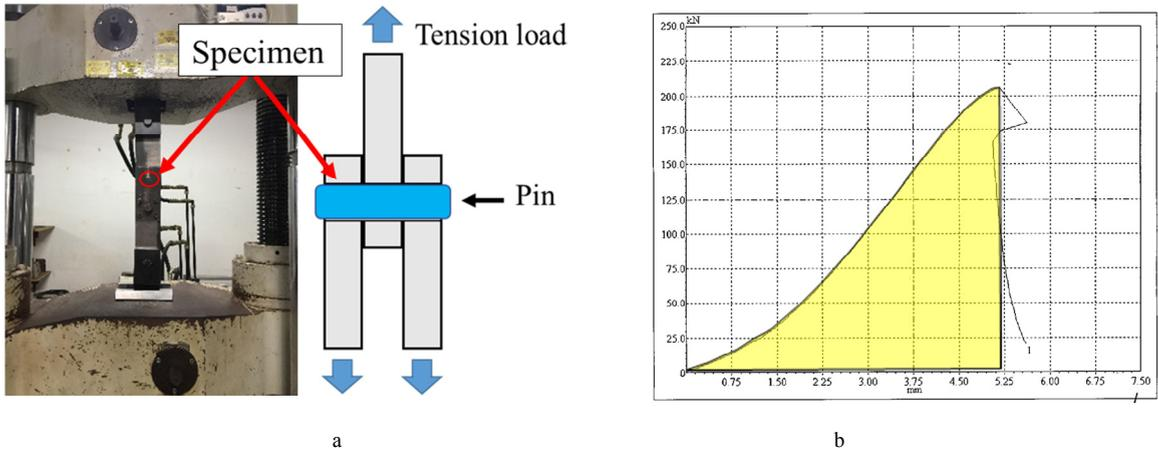
Fig. 6. (a) double shear test machine and specimen holder equipment; (b) double shear test result.
