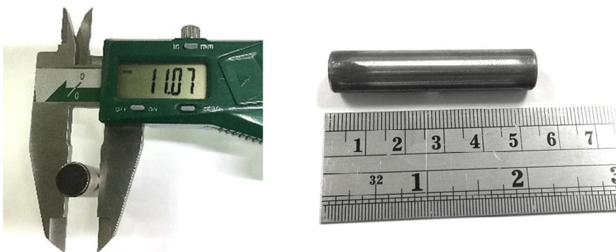
Fig. 2. Size of specimens.
