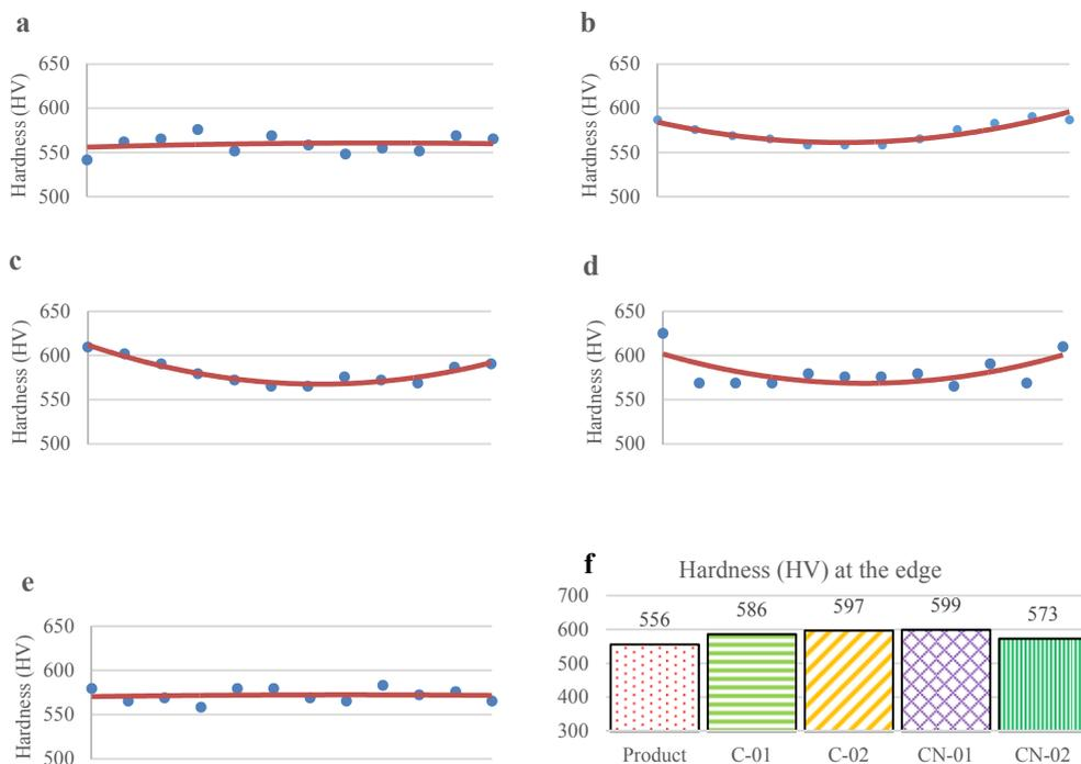
Fig. 8. Hardness profiles of (a) original product, (b) C-01, (c) C-02, (d) CN-01, (e) CN-02; (f) Comparison of Vickers hardness at the edge point of original product and experiment specimens.
