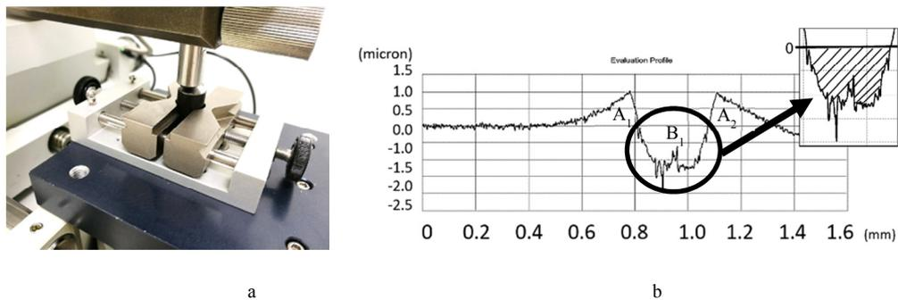
Fig. 7. (a) Pin-on-disk test; (b) Cross section area measured by surface roughness measurement device.
