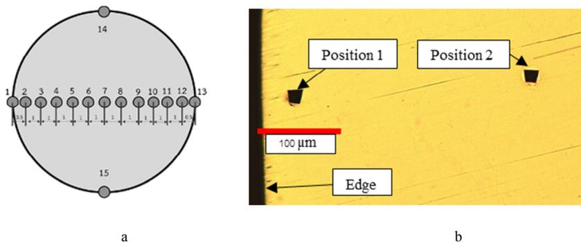
Fig. 5. (a) Position measurement of specimen; (b) Vickers hardness test points on the specimen.
