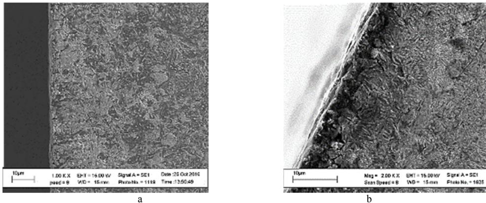
Fig. 11. Microstructure of (a) the original product and (b) the experiment specimen CN-01.
