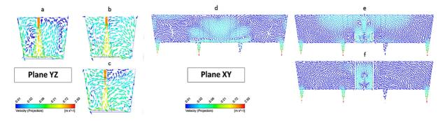
Fig. 5. Velocity flow field on the plane YZ of (a) bare tundish (b) tundish with dam and (c) tundish with baffle; Velocity flow field on the plane XY of (d) bare tundish (e) tundish with dam and (f) tundish with baffle.
