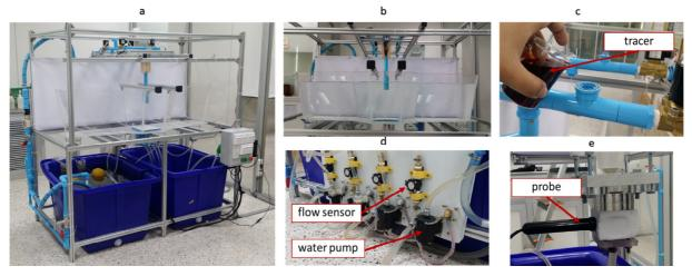
Fig. 4. Experimental setup of (a), (b) the physical water model of multi-strand tundish, (c) tracer, (d) flow sensor and water pump, (e) tracer measured probe.
