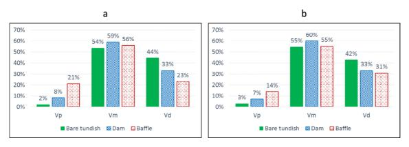
Fig. 9. Volume fraction of the flow in all tundish models obtained from (a) CFD simulation, (b) the physical water model.
