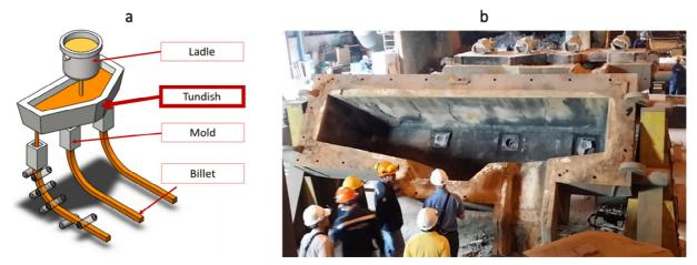
Fig. 1. (a) Diagram of continuous casting process. (b) The 4-strand tundish at Millcon Steel PLC, Thailand.
