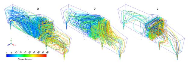
Fig. 6. Streamlines in (a) bare tundish, (b) tundish with dam and (c) tundish with baffle.
