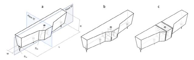
Fig. 2. Geometry of the tundish model with and without flow modifiers: (a) bare tundish, (b) tundish with dam and (c) tundish with baffle.
