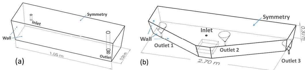
Fig. 2 Geometry and boundary conditions of (a) 1-strand, (b) 3-strand tundish models.
