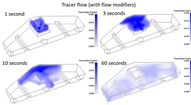
Fig. 6 The mass fraction of the tracer mixed the molten steel at various time after a pulse injection.
