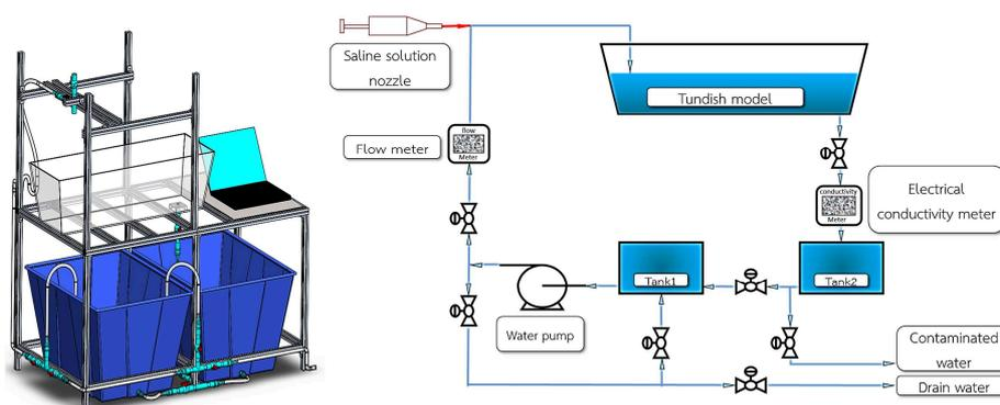
Fig. 8 The design of the laboratory scale physical water model for the future work.
