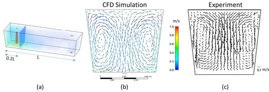
Fig. 3(a) Position of the observed plane, (b) Numerical result from the current study (c) Experimental result from the article. [6]
