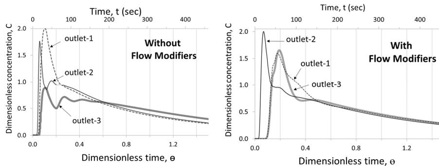
Fig. 7 Residence time distribution for each outlet of the tundish model (left) without flow modifiers and (right) with flow modifiers.
