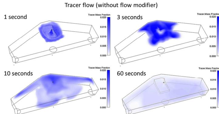
Fig. 5 The mass fraction of the tracer mixed with the molten steel at various time after a pulse injection.
