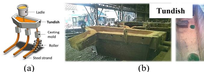
Fig. 1(a) Diagram of continuous casting process, (b) The 3-strand continuous casting tundish in the steelmaking shop at BSI, Thailand. [1]
