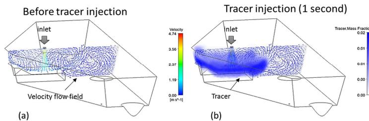
Fig. 4 (a) The steady state velocity flow field on the plane at the inlet position, (b) mass fractions of the tracer (blue color) mixed in the molten steel volume after a pulse injection.
