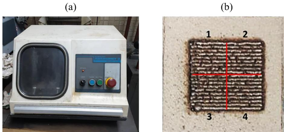
**Figure 3.16 The process of cutting the specimens, (a) cutting machine, (b) The cut specimens**
