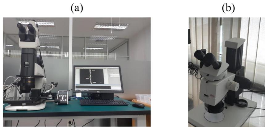
**Figure 3.15 The analysis equipment (a) Stereomicroscope, (b) macro camera**
