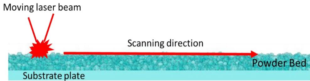
**Figure 3.6 The schematic of the powder bed and scanning direction of moving laser beam**
