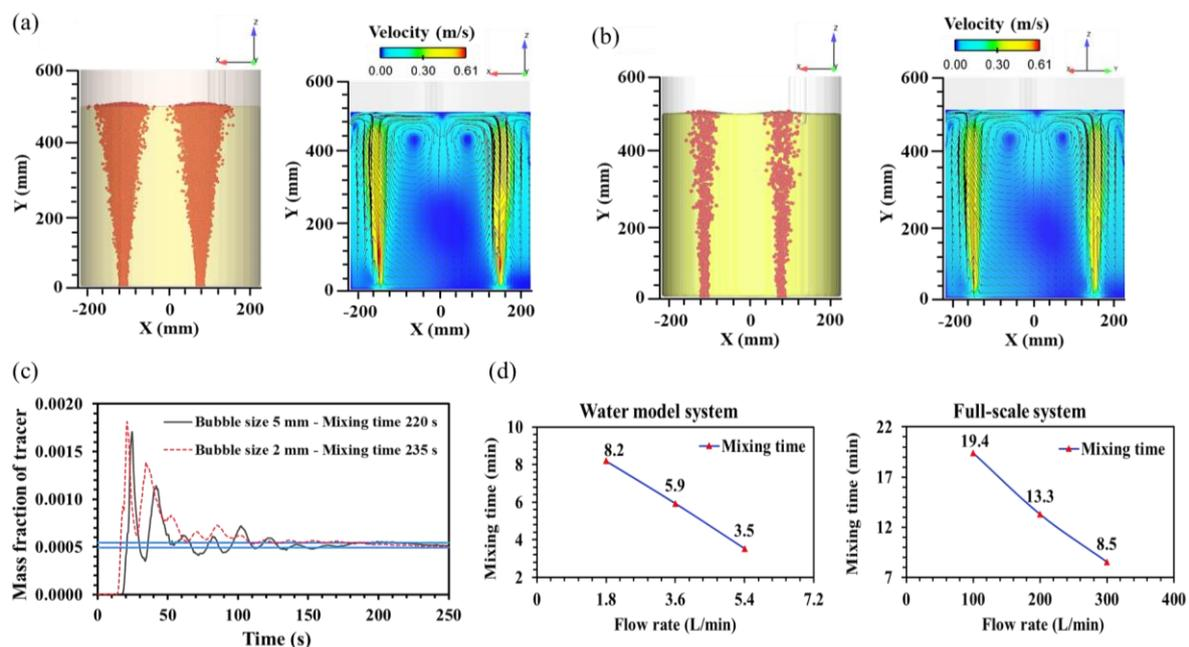
**Figure 2.** The results from the simulation; Plume regions and the velocity flow field of the bubbles with diffusion coefficient (a) 2 mm, (b) 5 mm, (c) 95% mixing time curve comparing between 2 mm and 5 mm bubble, (d) The mixing time from water model and full-scaled (steel-argon) systems
