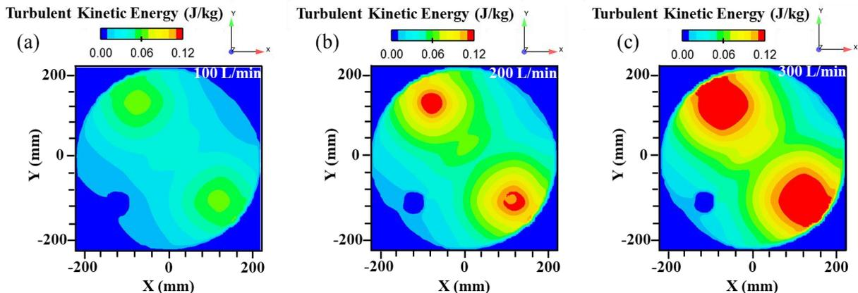
**Figure 3.** The turbulent kinetic energy with different flow rates from a full-scaled (steel-argon) system
