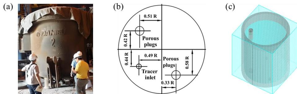
**Figure 1.** Geometric model of the ladle: (a) The full-scaled ladle furnace, (b) Arrangement of porous plugs and the tracer inlet and (c) Meshing model
