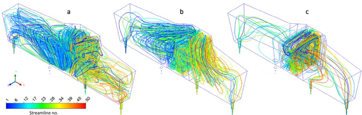
Fig. 6. Streamlines in (a) bare tundish, (b) tundish with dam and (c) tundish with baffle.
