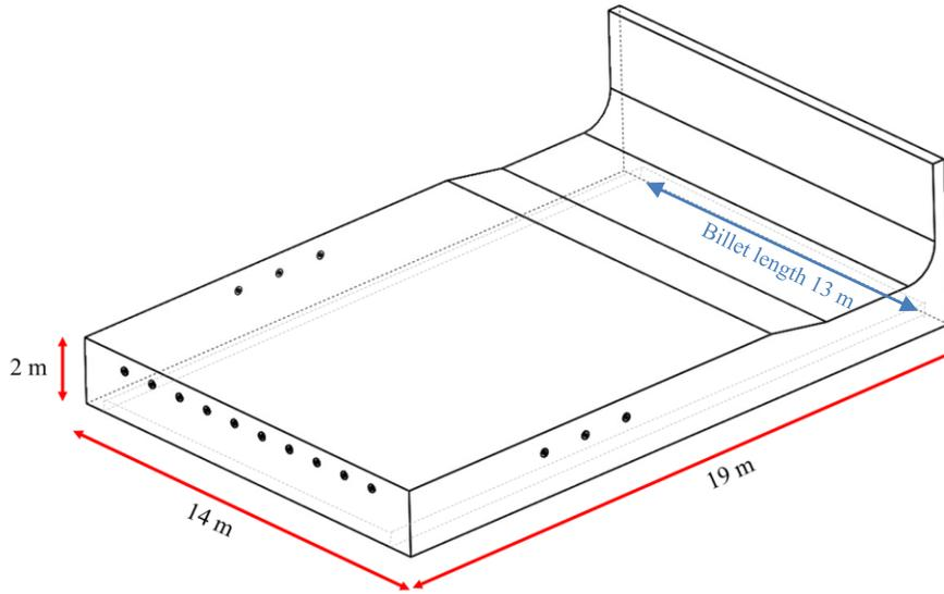
**FIGURE 2.** The 3D CAD model of reheating furnace
