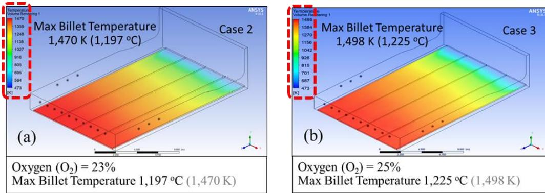
**FIGURE 5.** The simulation results of billet temperature: (a) 23% oxygen enrichment and (b) 25% oxygen enrichment
