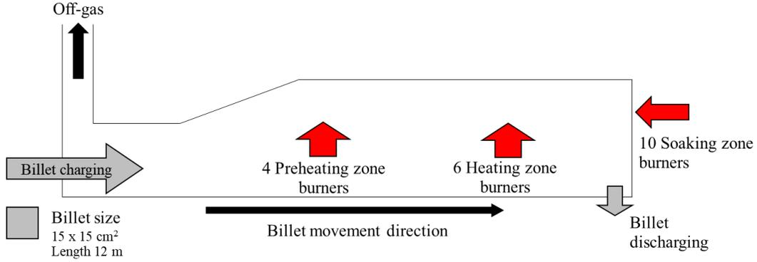
FIGURE 1. Schematic of reheating furnace operating in the example steel plant, Bangkok Steel Industry PCL
