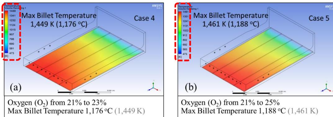
**FIGURE 6.** The simulation results of oxygen enrichment:
