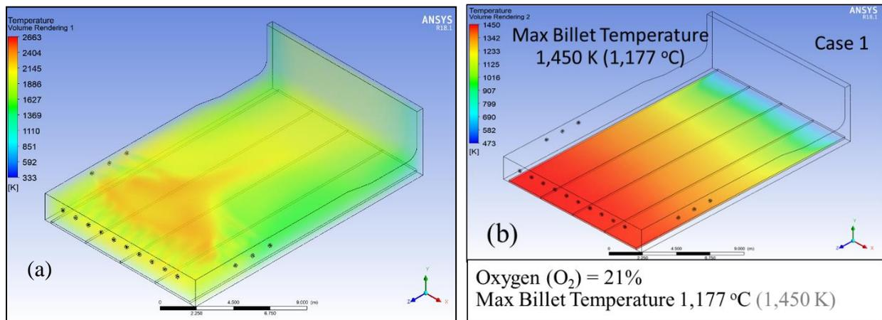
**FIGURE 4.** The simulation results of: (a) the reheating furnace and (b) the billet in case 1
