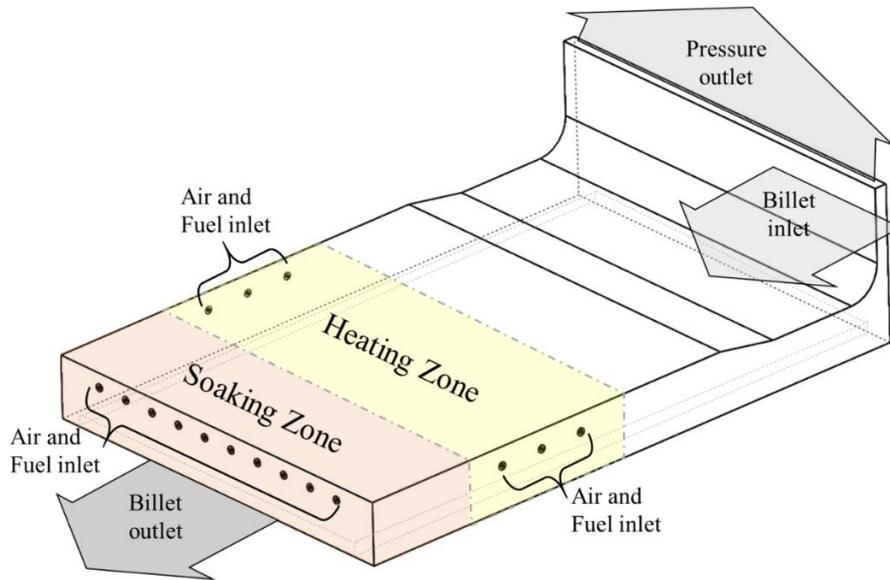
**FIGURE 3.** Boundary conditions of the reheating furnace
