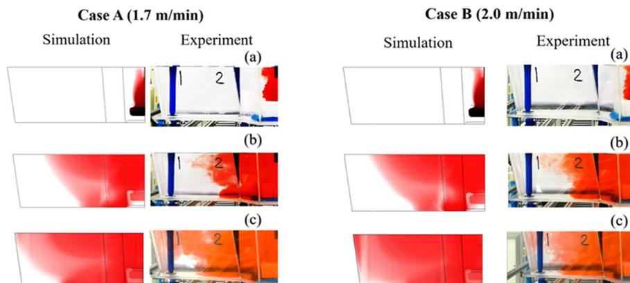
**Fig. 8.** The comparison of simulation results and experimental results with different casting speeds Case A (1.7 m/min); and Case B (2.0 m/min) after (a) 1; (b) 20 and (c) 50 s.
