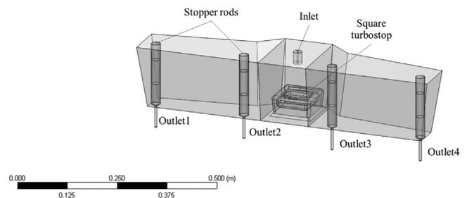
Fig. 2. Geometry of four strand tundish showing all components of tundish.
