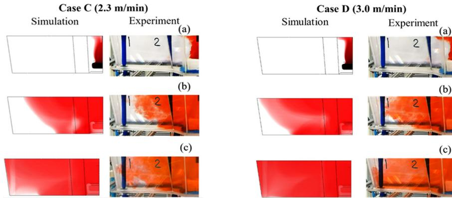
**Fig. 9.** The comparison of simulation results and experimental results with different casting speeds Case C (2.3 m/min); and Case D (3.0 m/min) after (a) 1; (b) 20; and (c) 50 s.
