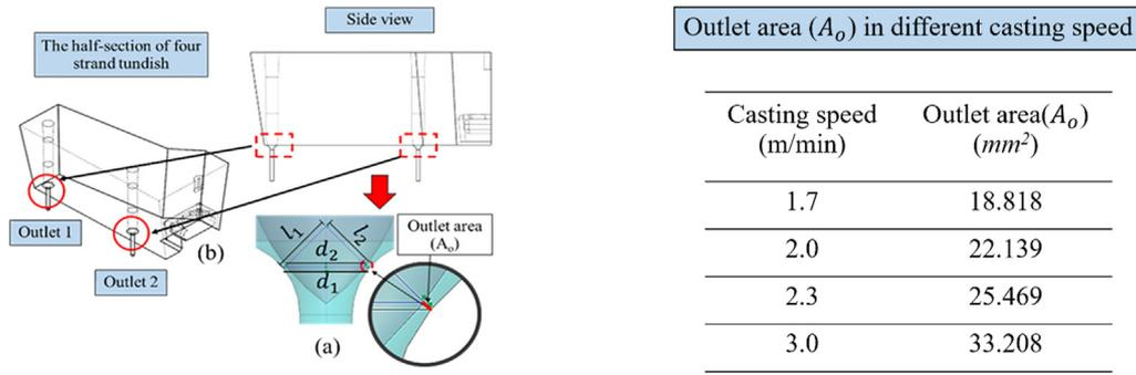
**Fig. 3.** (a) outlet's positions and the calculation of stopper rod lift in different casting speed; (b) the calculation of outlet area.
