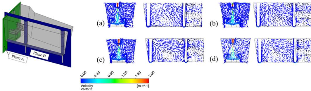
**Fig. 6.** The velocity flow field in the tundish with flow modifiers with different casting speeds of (a) case A; (b) case B; (c) case C and (d) case D.
