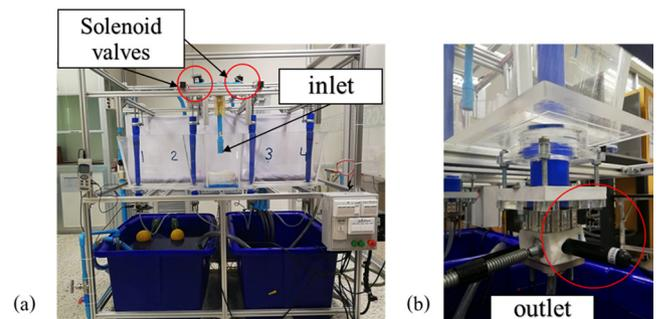
**Fig. 5.** (a) The physical water model and the solenoid valve; (b) the detection of conductivity.
