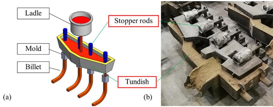
Fig. 1. (a) Schematic of continuous casting process; (b) The example of real tundish at example plant.
