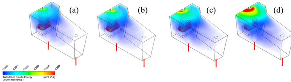
**Fig. 7.** Turbulence kinetic energy of different casting speeds at (a) case A; (b) case B; (c) case C and (d) case D.
