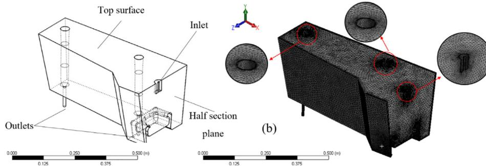
**Fig. 4.** (a) Boundary conditions; (b) the computational mesh in the half-section tundish.
