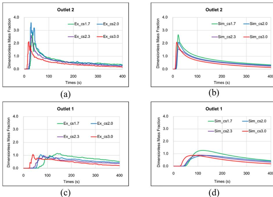
**Fig. 10.** RTD curves obtained from experimental results at (a) mid-outlet; (c) far-outlet; RTD curves obtained from the simulation results at (b) mid-outlet; (d) far-outlet.
