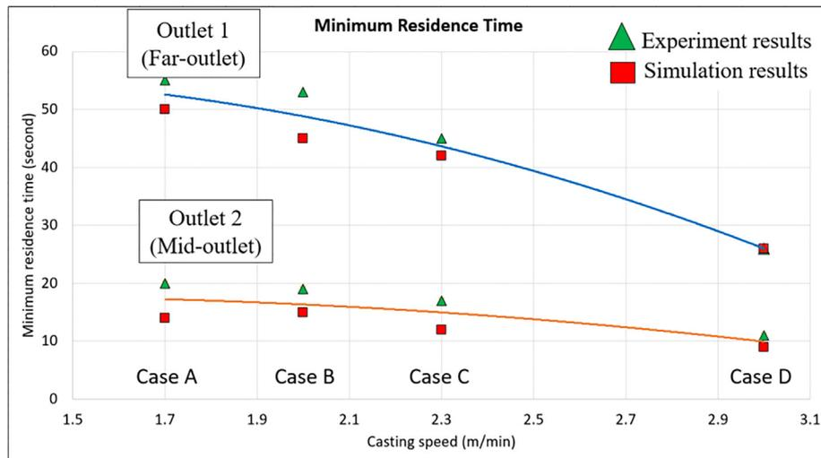
Fig. 11. . The minimum residence time of tracer in all cases between experiment and simulation results.
